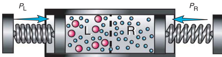
Fig. 1.4 Physical origin of osmotic pressure. The two compartments, L and R, are separated by a semi-permeable wall, represented by the broken line. The two walls at the ends of the compartments are movable (and can be thought of as the stretchable membranes of “cells” L and R) and attached to springs, which measure the pressure in L and R. The larger, pink particles (the solute) cannot pass through the wall in the middle, but the smaller blue particles (the solvent) can. At equilibrium the pressure exerted by the solvent on the movable walls in L and R is the same. If the two compartments contain the larger particles at different concentrations (in the figure their concentration in R is zero), the pressures they exert on the movable walls are not equal: their difference is called the osmotic pressure. In particular, if the two springs are made of the same material, the one attached to L will be more compressed, corresponding to the membrane of “cell” L being more stretched.
